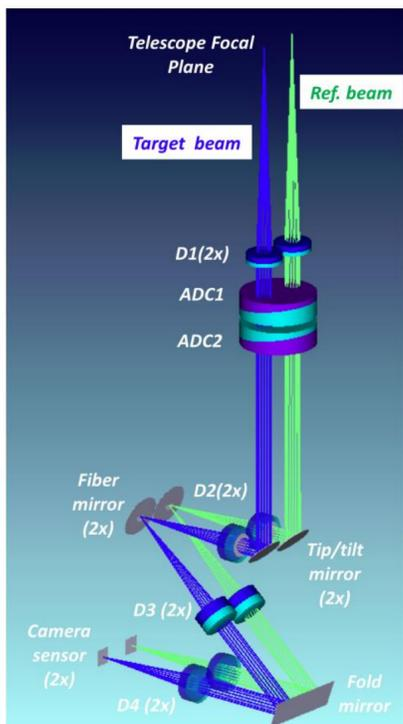
Figure 2: Optical schematic of the Cassegrain Fibre Adapter System.
