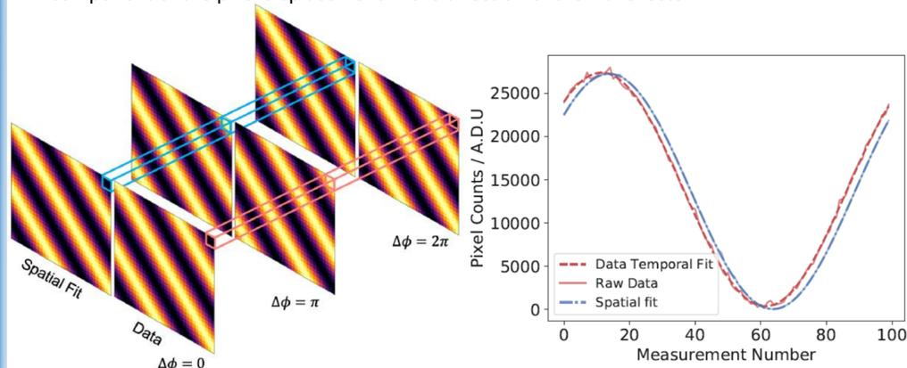
Figure 3: (Left Panel) Image demonstrating the fringes imaged over the CCD with the interference pattern scanned over a  $2\pi$  phase change. (Right Panel) Plot of measurement number over a  $2\pi$  phase change against counts detected by the pixel for both the data collected by the pixel and the spatial fit of the fringes for the whole CCD; the difference in their phase holds position information.
