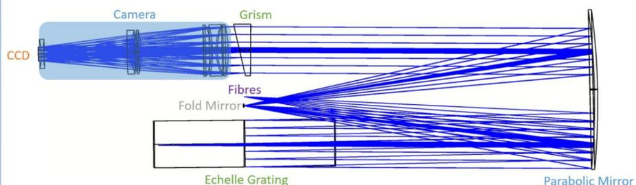
Figure 1: Annotated optical schematic of the HARPS3 Spectrograph.
